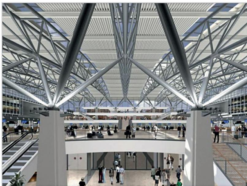
Figure 17: Building with Tubular Structures, Column Trees and "Banana" Trusses, Source: Civil.IITB
